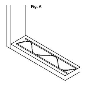
Apply a continuous  $\frac{3}{16}$  – 1/4" bead of silicone caulk around exterior face of rough opening, about  $\frac{1}{2}$ " from edge to MAINTAIN A PERMANENT SEAL between sheathing and nailing fins.
